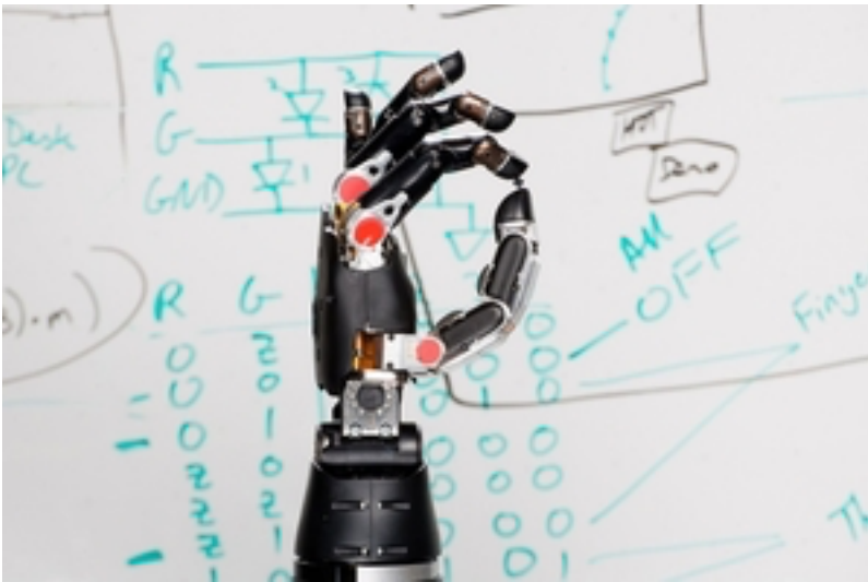
One of the most advanced prosthetic hand. It connects with the brain taking commands from it and feeding back touch sensations. Credit: John Hopkins University
