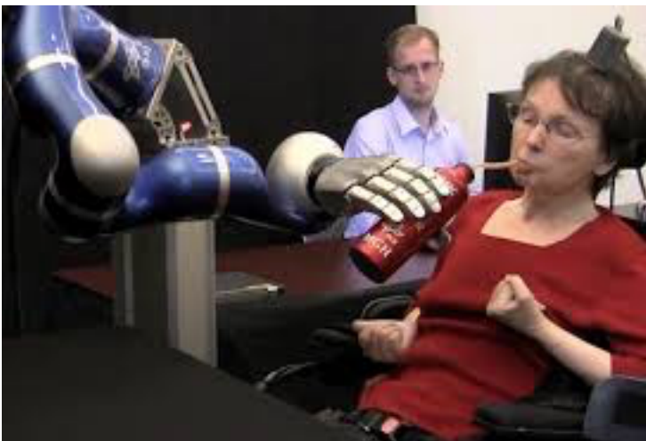
A 58-year-old woman, paralysed by a stroke for almost 15 years, uses her thoughts to control a robotic arm, grasp a bottle of coffee, serve herself a drink, and return the bottle to the table. Credit: Brown University – 2012
